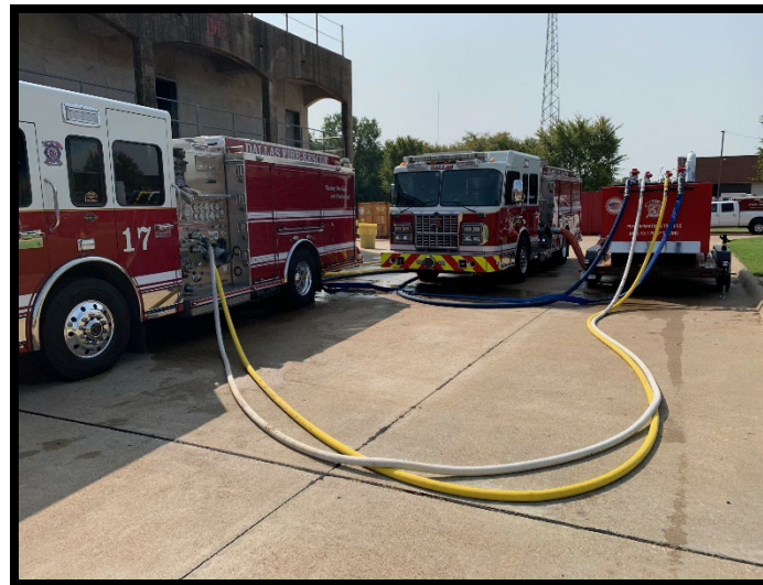
Fire Training Center closed loop pump simulator
