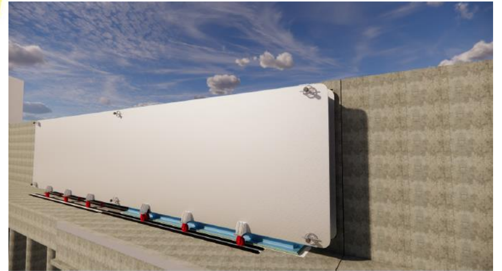
View of typical concept of Roller Gate
